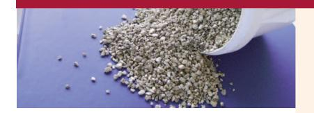
Natural product of volcanic origin, based on their performance absorbent capacity of the expanded vermiculite back with repellent treatment, very light material, with high buoyancy and chemical affinity for oils and hydrocarbon.
