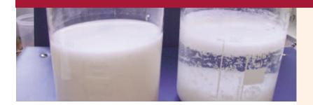
Solid product easily soluble in water of high molecular weight, specific for the clarification of industrial waters, separation of solids in mining, treatment of water of cabins of paints and industrial processes.
